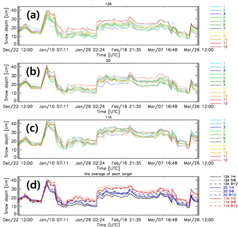
**Figure 3.** Time series of snow depth from snow stakes on base (a) 12A, (b) 20, and (c) 11A from manual observations over the period from 22 December 2013 to 26 March 2014. The line colors indicate individual snow stakes. (d) Average snow depth of four snow stakes on same snow depth target. The line color indicates each base. The solid, dotted, and dashed lines represent average snow depth of stake numbers 1–4, 5–8 and 9–12 on the same snow depth target.
