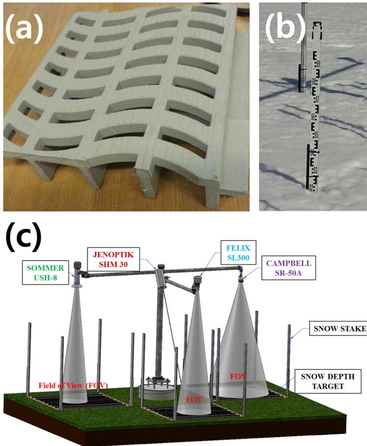
**Figure 2.** Snow depth measurement system. **(a)** Grey plastic decking comprising snow depth target, **(b)** wooden snow stake, and **(c)** installation of snow depth sensors for base 11A (courtesy: Environment Canada).
