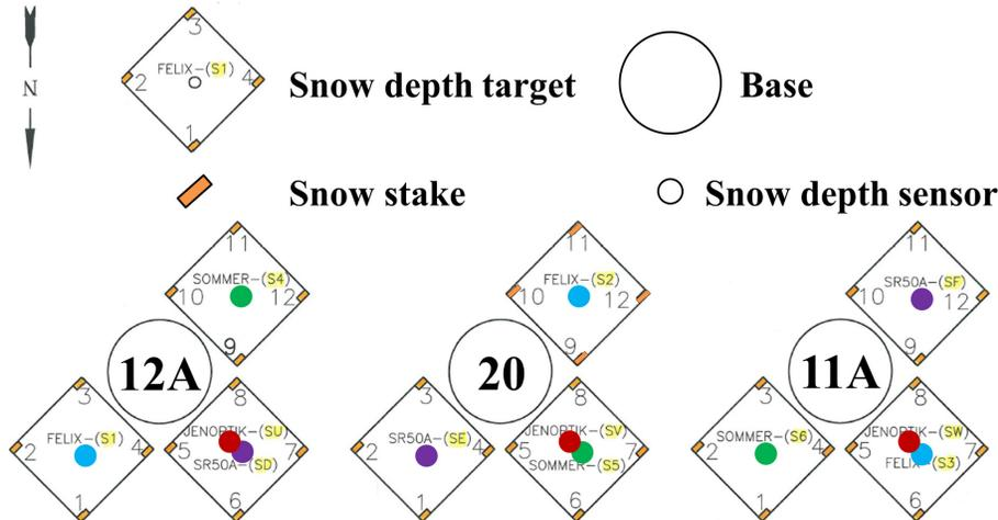
**Figure 1.** Layout of snow depth measurement system at the CARE site during the 2013–2014 winter season. The large circles (squares) represent bases (snow depth targets). The orange rectangles and small circles indicate snow stakes and snow depth sensors, respectively (courtesy: Environment Canada).
