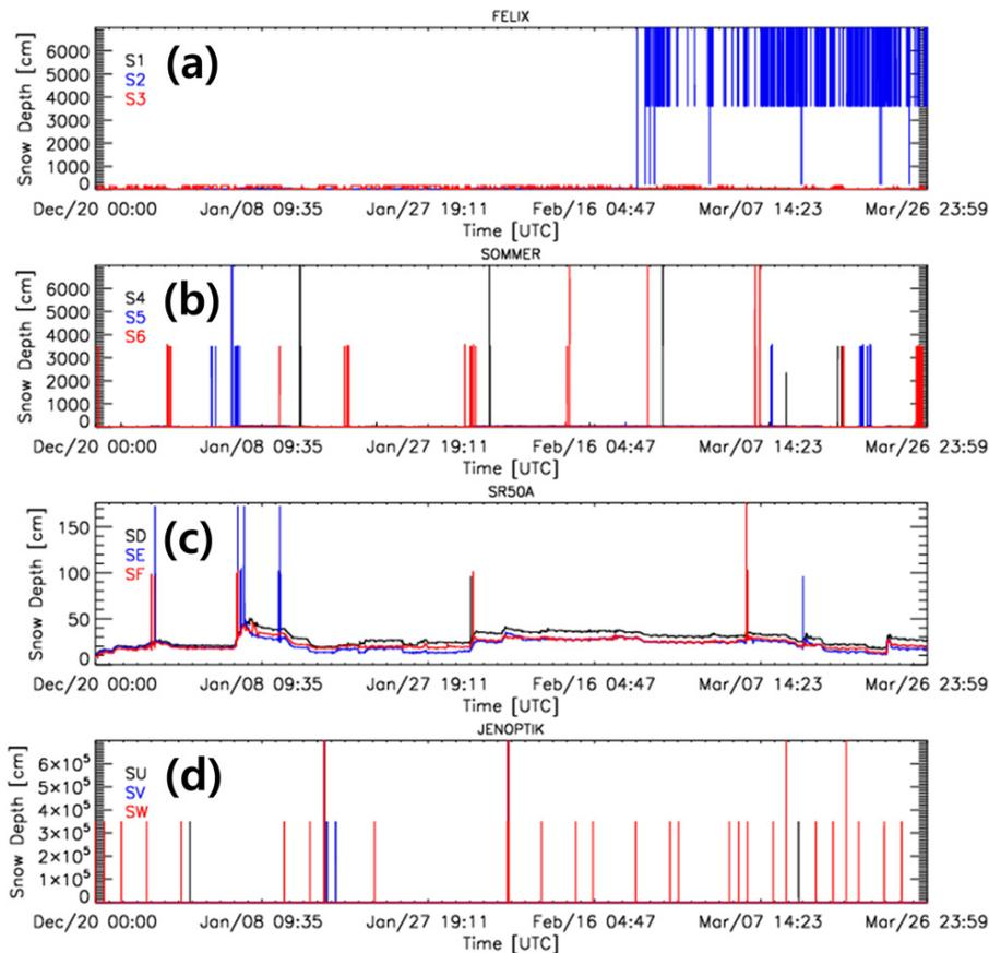
**Figure 5.** Time series of snow depth from (a) FEL, (b) SOM, (c) SR50A, and (d) JEN for the period from 20 December 2013 to 26 March 2014. The black color indicates sensors on base 12A. The blue color indicates sensors on base 20. Finally, the red color indicates sensors on base 11A.
