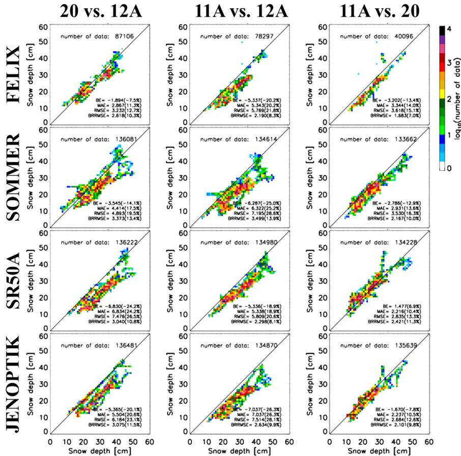
**Figure 11.** Scatter plots of snow depth measured by two snow depth sensors of the same type on bases 20 vs. 12A (left), 11A vs. 12A (middle), and 11A vs. 20 (right): FELIX (first column), SOMMER (second column), SR50A (third column), JENOPTIK (fourth column). The values in brackets indicate the NBE, NMAE, NRMSE, and NBRMSE.
