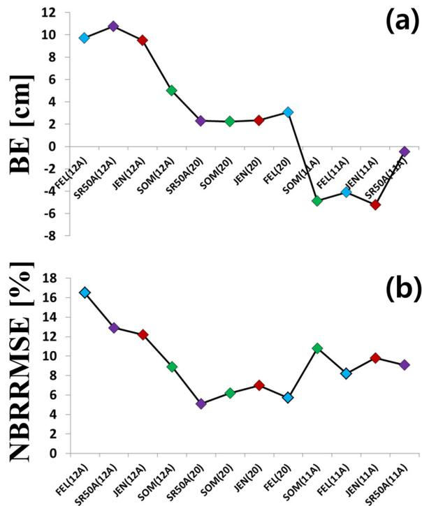
**Figure 10.** (a) BEs and (b) NBRMSEs of each snow depth sensor. The blue, purple, red, and green diamonds represent FEL, SR50A, JEN, and SOM.
