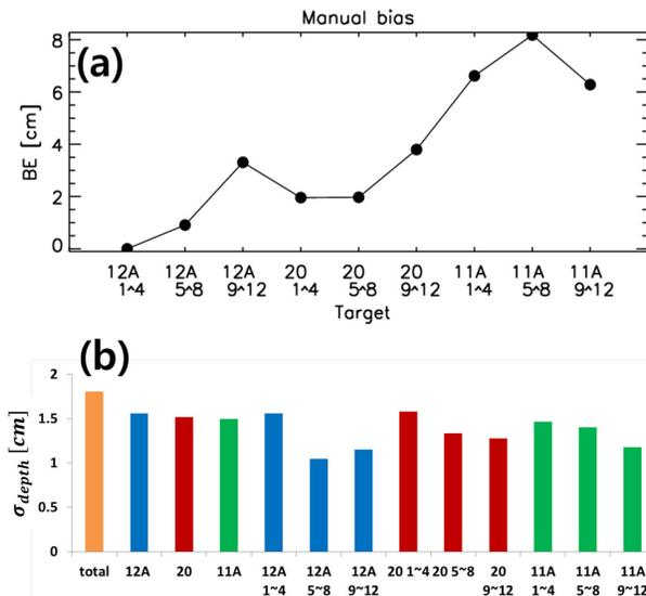
**Figure 8.** (a) BEs and (b) uncertainties of manual snow depth measurements. The BEs are calculated for each snow depth target. The orange bar represents the  $\sigma_{depth}$  for all pairs. The 2nd–4th (5th–13th) columns indicate the  $\sigma_{depth}$  for each base (snow depth target). The color of bars indicates the same base; the blue, red, and green bars represent  $\sigma_{depth}$  for bases 12A, 20, and 11A.
