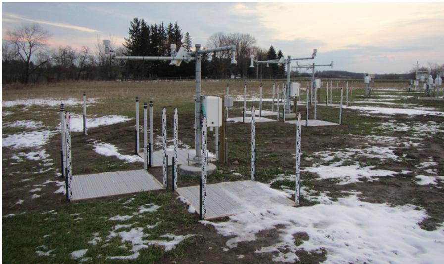
**Figure 4.** Photograph of the uneven snow deposition on the surface of snow depth targets.
