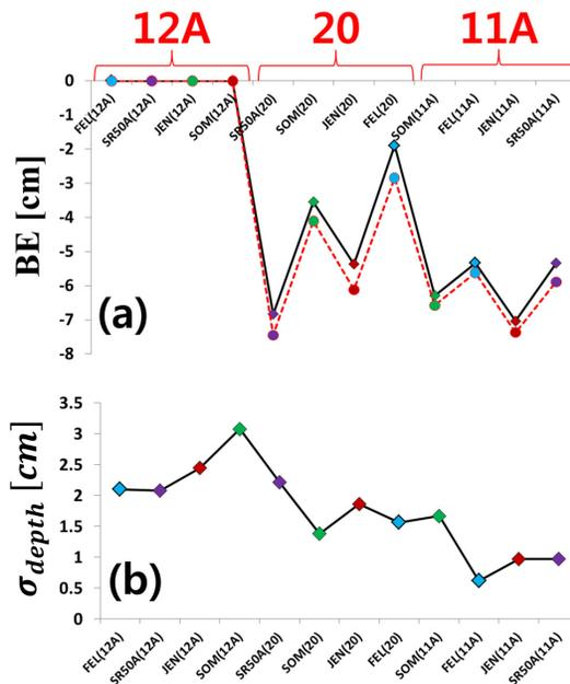
**Figure 12.** (a) BEs of each snow depth sensor. The diamonds (circles) are calculated by considering the snow depth sensors on base 12A as reference (the BEs in Figs. 8a and 10a are added and snow depth from snow depth sensor on base 12A are then used as reference). (b)  $\sigma_{\text{depth}}$  of each snow depth sensor. The blue, purple, red, and green diamonds indicate FEL, SR50A, JEN, and SOM.
