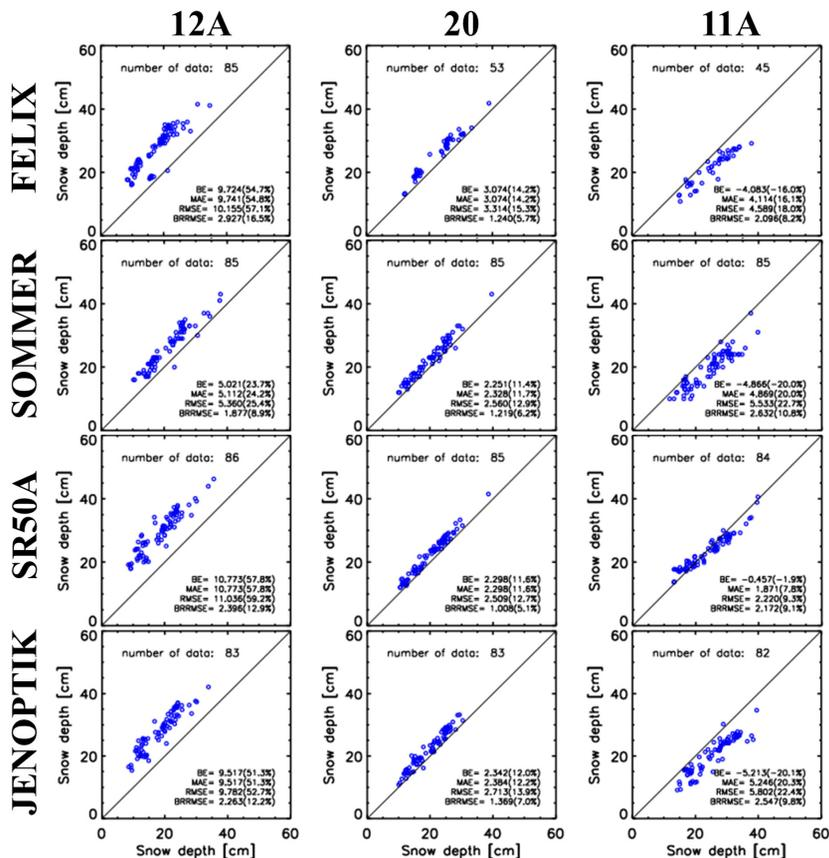
**Figure 9.** Scatter plots of snow depth measured by automatic snow depth sensors (y axis) and average snow depth of manual observation (x axis) on bases 12A (left), 20 (middle), and 11A (right): FELIX (first column), SOMMER (second column), SR50A (third column), and JENOPTIK (fourth column). The values in brackets indicate the NBE, NMAE, NRMSE, and NBRMSE.
