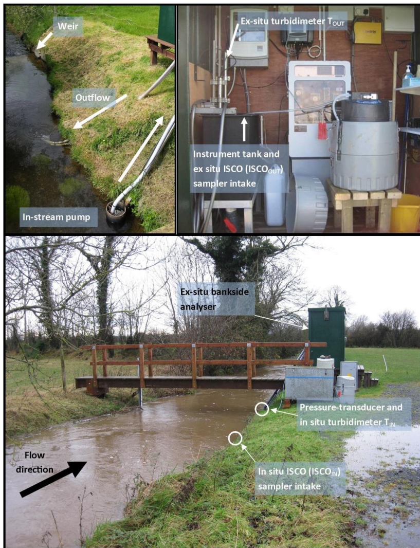
Figure 2: Picture of in situ and ex situ suspended sediment and discharge instrumentation at Grassland B.
