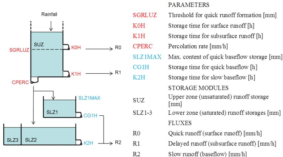
**Figure 5.** Runoff generation module of PREVAH, adapted from Viviroli et al. (2009). Parameters in blue are averaged for the whole catchment, while parameters in red are adapted stepwise to the RTs.
