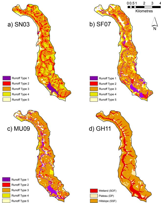
**Figure 4.** DRP-maps for the Reppisch catchment: **(a)** reference map according to Scherrer and Naef (2003) and automatically derived map according to **(b)** Schmocker-Fackel et al. (2007); **(c)** Müller et al. (2009); **(d)** Gharari et al. (2011).
