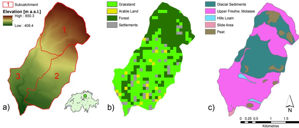
**Figure 1.** Overview of the Meilen catchment, Switzerland. **(a)** Digital Terrain Model (25 m resolution) subdivided into 3 sub-catchments; **(b)** land-use map (100 m resolution); **(c)** geology map (data: BFS GEOSTAT/Federal Office of Topography swisstopo).
