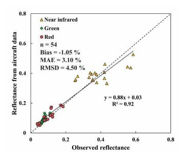
**Figure 2.** Comparison between observed (*O*) and modeled (*M*) visible band reflectance. The statistics (for the sample size n=54) listed in the figure are the Bias ( $\Sigma$  (O-M)/n), mean absolute error (MAE= $\Sigma$ |O-M|/n) and root mean square difference (RMSD=[ $\Sigma$ (O-M)<sup>2</sup>/n]<sup>1/2</sup>) where the symbol  $\Sigma$  represents a summation over the sample size n.
