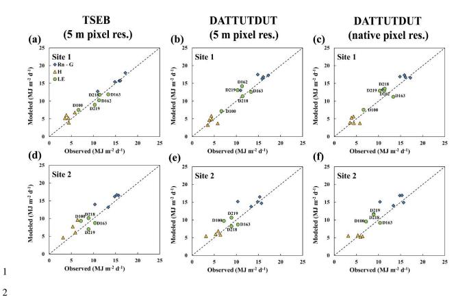
**Figure 7.** Scatter plot of observed and modeled daytime fluxes from (a) TSEB (5 m pixel resolution), (b) DATTUTDUT (5 m pixel resolution) and (c) DATTUTDUT (native pixel resolution) for the five days in 2013. The observed energy components are adjusted for energy balance using the RE method.
