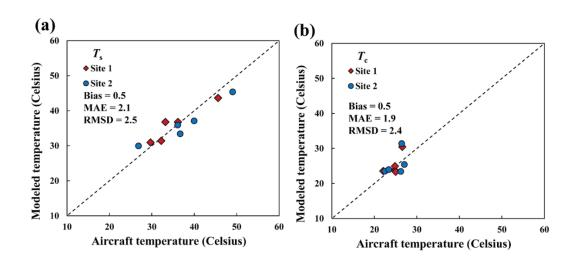
**Figure 5.** Comparison between modeled  $T_s$  and  $T_c$  from TSEB and values extracted from the aircraft imagery on the five acquisition days. All the statistics (Bias, MAE and RMSD) have units of  $\mathbb{C}$ .
