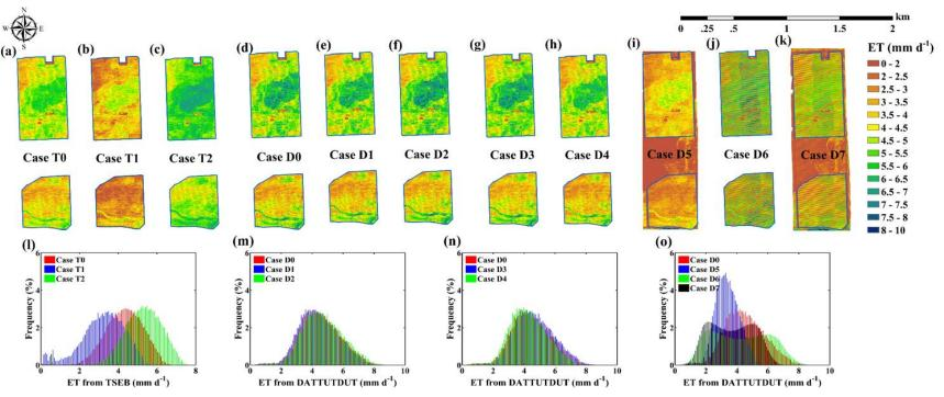
**Figure 10.** Comparison of the ET patterns and frequency distributions generated by TSEB and DATTUTDUT under the sensitivity tests described in Table 6.
