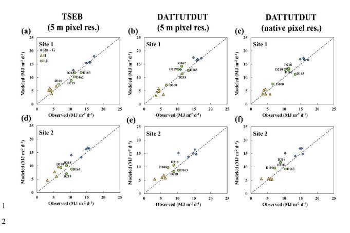
Figure 7. Scatter plot of observed and modeled daytime fluxes from (a) TSEB (5 m pixel resolution), (b) DATTUTDUT (5 m pixel resolution) and (c) DATTUTDUT (native pixel resolution) for the five days in 2013. The observed energy components are adjusted for energy balance using the RE method.
