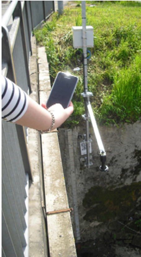
Figure 1. Example of a low-cost social sensor, and crowdsourced observations, implemented in the Bacchiglione river, Italy, under the WeSenseIt project.
