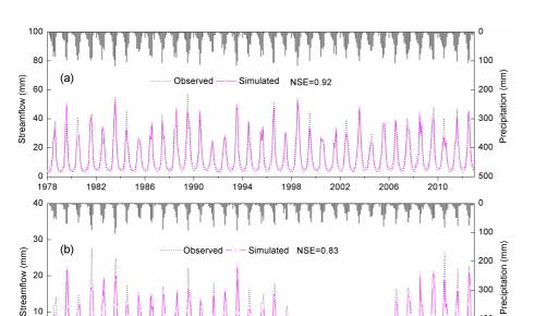
Figure 4. Time series of observed and simulated monthly streamflow using the abcd model in the Region I (a) and Region II (b) during 1978-2012.
