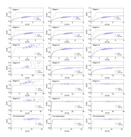
**Figure 8.** Comparison of the original Budyko curves (left panel) and the new *Fu*-type Budyko curves (middle panel, with  $\lambda = 0$ ) and the new *Fu*-type Budyko curves (right panel, with  $\lambda > 0$ ) for Regions I–VI and the whole basin at the annual time scale.
