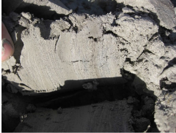
Figure 8 Fine sand sample with thin silty laminas from test field SF/SU1 (see Fig. ( 7))
