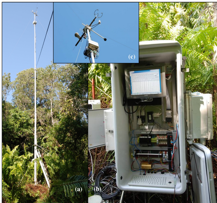
Figure 2. (a) Telescopic mast (21.3 m) erected in the swamp forest to raise the eddy covariance instruments above the forest canopy, (b) the computer installed at the swamp forest, housed in a temperature controlled enclosure and (c) the instruments attached to the head of the mast.
