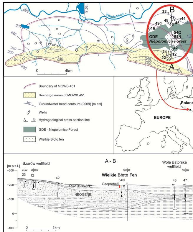
**Figure 1.** Hydrogeological map and cross-section of the Bogucice Sands (Neogene) aquifer (Major Ground Water Basin – MGWB 451). The study area is marked by ~~brown-red~~ red oval. Open circles mark the position of pumping wells. Cross-section according to Górká et al. (2010).
