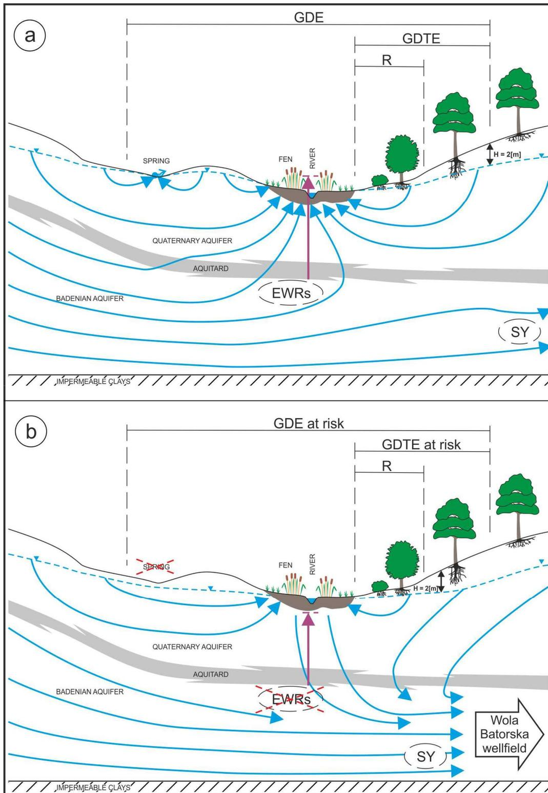
**Figure 3.** Conceptual model of the Wielkie Bloto fen. **(a)** - natural state; **(b)** - envisaged future status as a result of intense exploitation of the Wola Batorska wellfield. GDE - Groundwater Dependent Ecosystem; GDTE - Groundwater Dependent Terrestrial Ecosystem, R – riparian forest, EWRs - Environmental Water Requirements, SY – Safe Yield of the aquifer exploited by the Wola Batorska wellfield.
