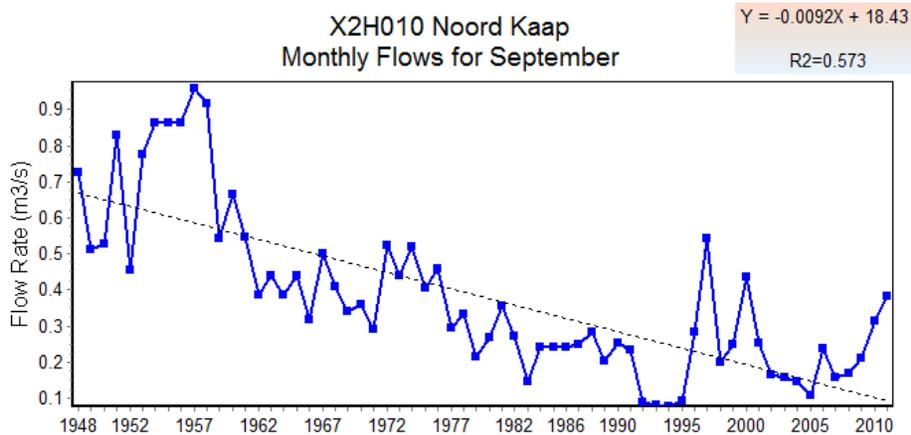
**Figure 9.** Plot of median monthly flows for September for the entire time series (1949–2011) on the Noord Kaap Gauge, located on the Crocodile sub-catchment.
