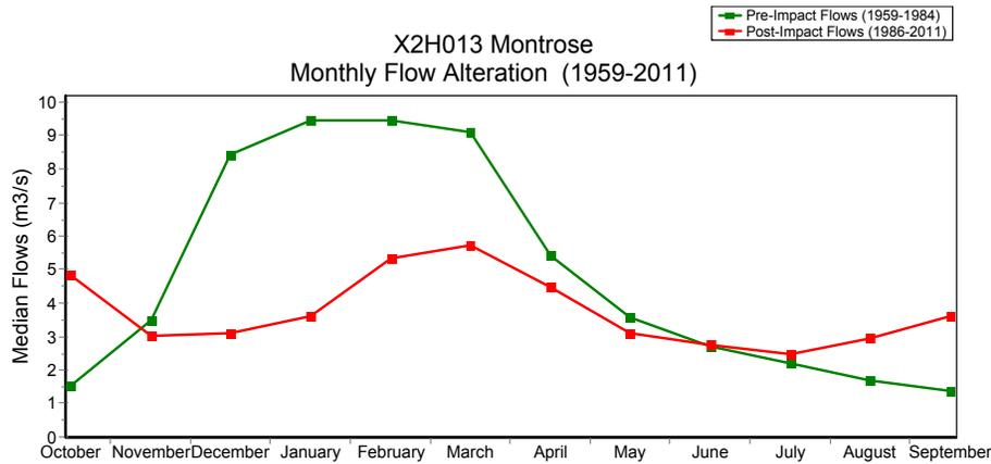
**Figure 11.** Impact of Kwena Dam (commissioned in 1984) on streamflows of the Crocodile River, Montrose Gauge X2H013.
