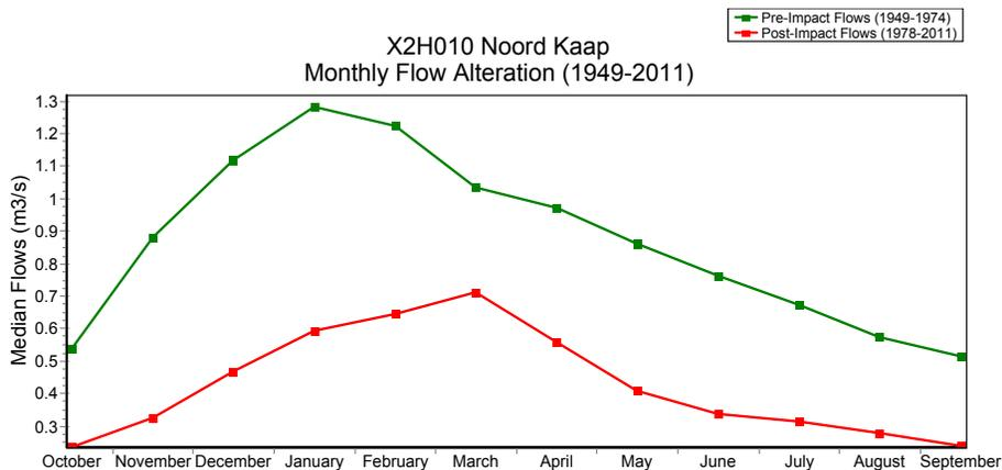
**Figure 10.** Plot of median monthly flows for 2 periods (1949–1974 and 1978–2011) on the Noord Kaap Gauge, located on the Crocodile sub-catchment.
