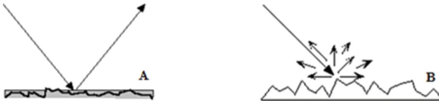
Fig. 8. (A) Specular reflection from flooded areas; (B) diffuse reflection from non-flooded area.
