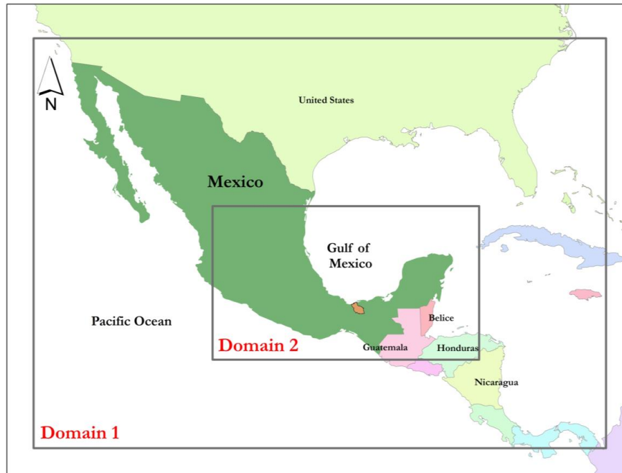
Figure 2. Numerical setup of the WRF with a nested domain covering Mexico. Domain 1: 25 km resolution; Domain 2: 4 km resolution; the orange region illustrates the Tonalá catchment.
