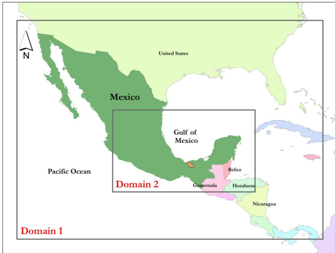
4 Figure 2. Numerical setup of the WRF with a nested domain covering Mexico. Domain 1: 5 25km resolution; Domain 2: 4km resolution; the orange region illustrates the Tonalá 6 catchment.
