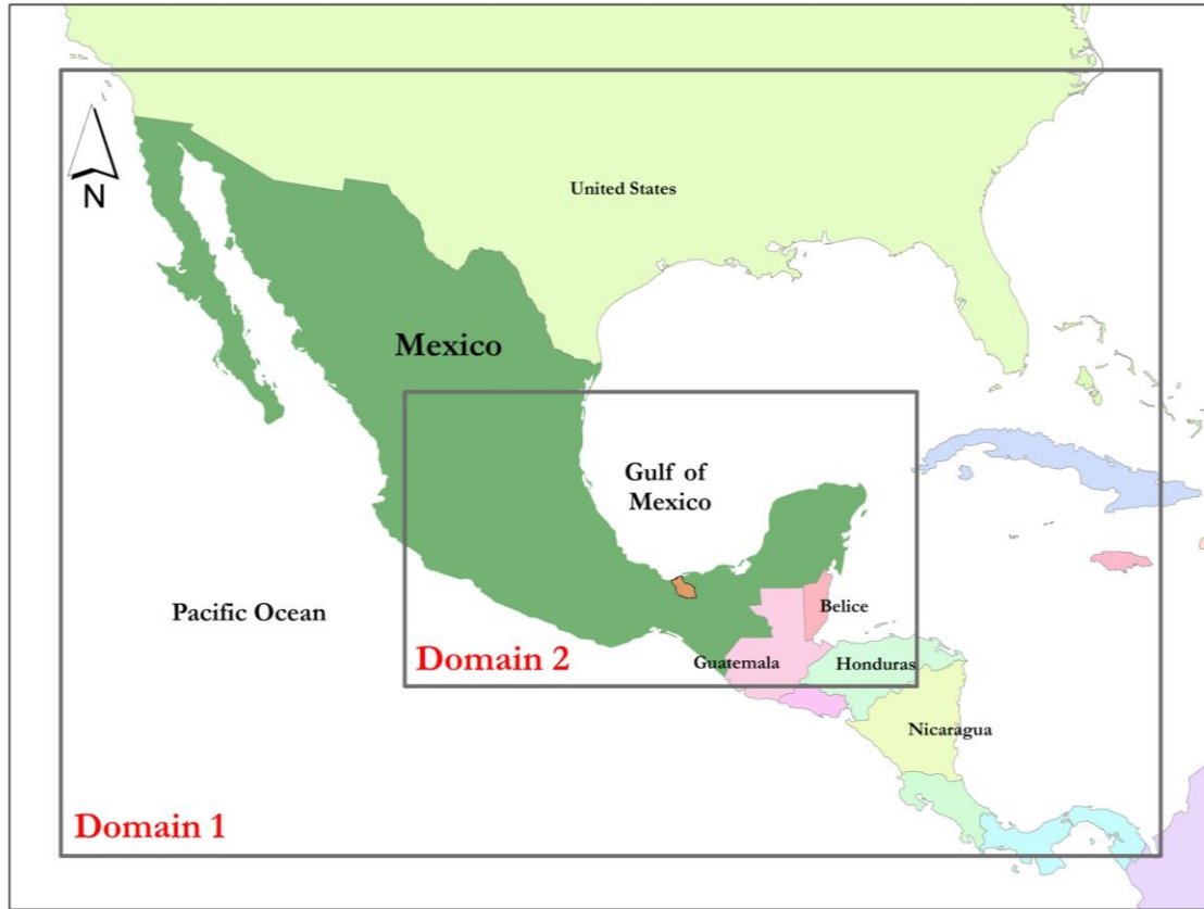
Figure 2. Numerical setup of the WRF with a nested domain covering Mexico. Domain 1: 25km resolution; Domain 2: 4km resolution; the orange region illustrates the Tonalá catchment.
