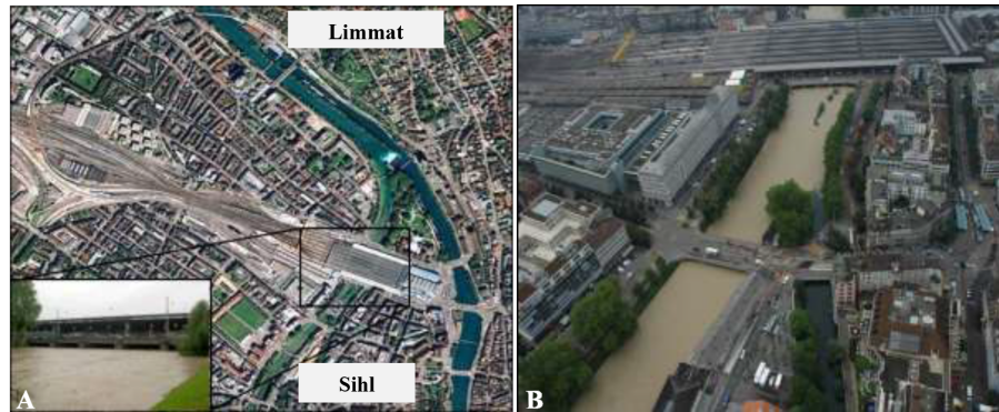
Figure 2. Sihl River flowing beneath Zurich main train station before it joins the Limmat River: (A) image adapted from Google map; the box at the bottom shows the critical Sihl River section in August 2005 during a flood even, source: A. Senn (WSL). (B) Sihl River flowing underneath Zurich main train station in August 2005 (discharge: 280 \text{ m}^3 \text{ s}^{-1} ), source: Office of Waste, Water, Energy and Air, Zürich (M. Oplatka).
