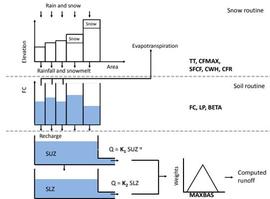
**Fig. 1.** Structure of the HBV model.
