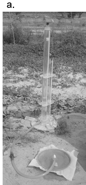
Figure 2. Photographs of some of the experimental measurement methods; (a) Disc infiltrometer; (b) Beerkan method; (c) Evaporation method.
