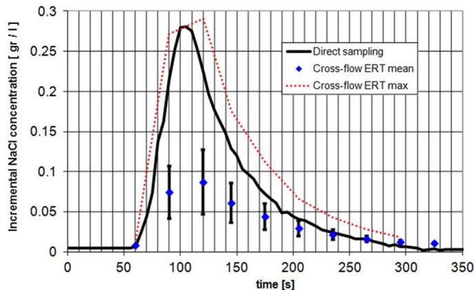
**Fig. 10.** Comparison of direct sampling and cross-flow FERT obtained concentration curves; the dashed red line refers to the maximum concentration value determined from cross-flow FERT in the area of the canal reported in Fig. 11.
