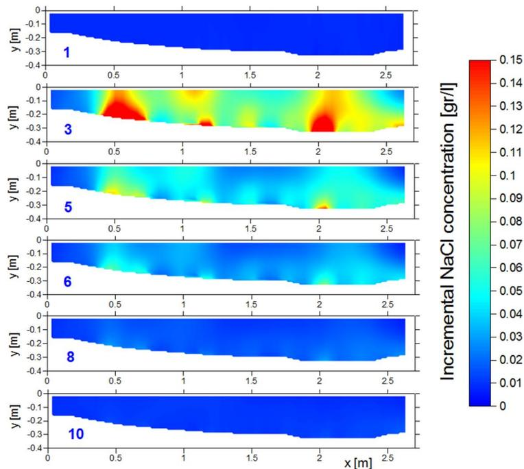
**Fig. 8.** Concentrations in the imaged section for increasing times, image number with reference to Fig. 6, seen from up-stream.
