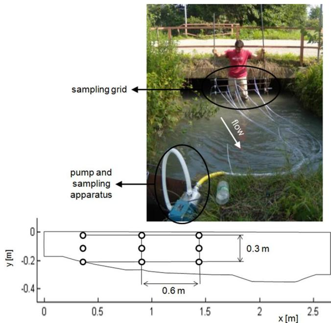
**Fig. 4.** Multi-sampling system with details of the sampling grid (black circles are water spilling points) and of the pumping apparatus; the below section is seen from up-stream.
