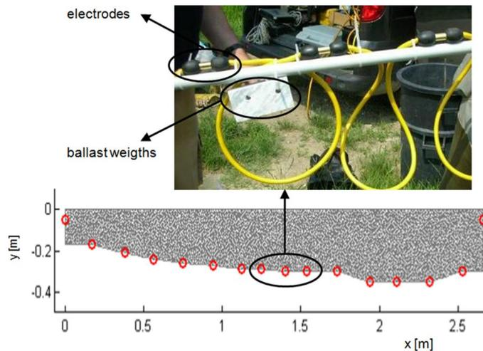
**Fig. 5.** Electrodes disposition for cross-flow FERT: images of the electrodes and the anchoring system (top panel) and of the mesh used for the inversion (bottom panel), the below section is seen from up-stream.
