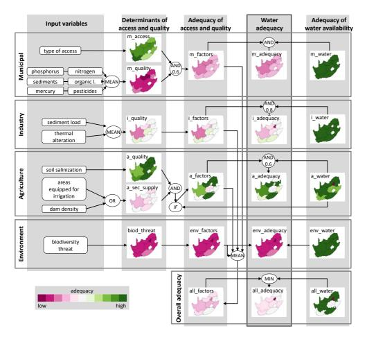
**Fig. 2.** Fuzzy aggregation tree to calculate the adequacy of available water resources. Maps show values for South Africa using water availability data from the GFDL-ESM2M model under current conditions (GDFLbase).
