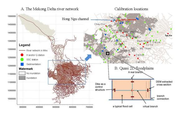
Fig. 2. (A) The model river network and the calibration locations. (B) Quasi-2-D concept for a typical floodplain compartment in the VMD.
