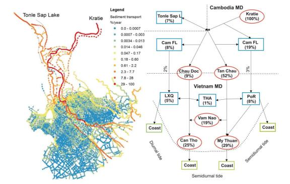
**Fig. 5.** Proportion of transported sediment in the whole MD compared to sediment load at Kratie (left panel). Sediment load transport into subsystems (green blocks) and to key stations (red circles) for the year 2009 (right panel).
