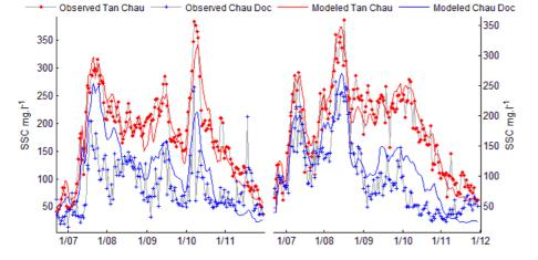
Fig. 4b. Comparison of measurements and simulation results at Tan Chau and Chau Doc: daily SSC for the calibration year 2011 (right panel) and for the validation year 2009 (left panel).
