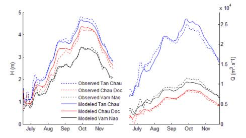
Fig. 4a. Comparison of measurements and simulation results at stations Tan Chau, Chau Doc and Vam Nao for 2011: daily water levels (left panel), daily discharges (right panel).
