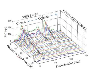
Fig. 7. Typical SSC reduction in the channels with distance to the main river in the Plain of Reeds, exemplarily shown for the Hong Ngu channel in 2011.
