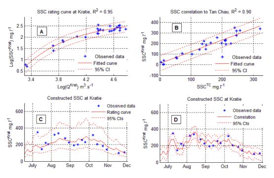
**Fig. 3. (A)** Derived SSC for Kratie using sediment rating curve, **(B)** derived SSC for Kratie using correlation to SSC at Tan Chau, **(C)** comparison of sediment rating curve method with measured data in 2011, **(D)** comparison of correlation method with measured data in 2011.
