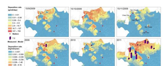
**Fig. 9.** Map of sedimentation in the VMD floodplains. Top panels: sediment deposition rate (gm<sup>-2</sup> day<sup>-1</sup>) during the period of compartment opening (left panel), during flood peak discharge (center panel) and during the period of compartment closing (right panel). Bottom panels: cumulative sediment deposition (kgm<sup>-2</sup> yr<sup>-1</sup>) in 2009, 2010 and 2011. The bars show the differences of cumulative sediment deposition between measurements and simulation.
