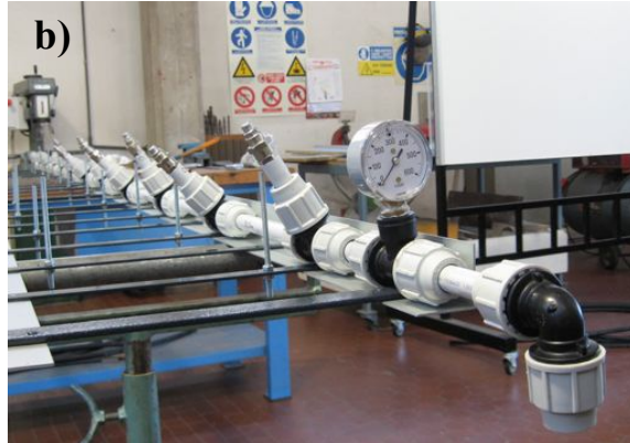
Figure 1. Nozzle line setup. (a) Nozzle assembly. The threaded pressure washing nozzle was connected to a short length of PVC pipe using two connectors. (b) Alternating angles of nozzles and pressure gauge used to regulate flow.
