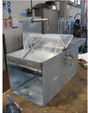
Figure 4. Tipping bucket flow gage. (a) Dimensions of the flow gage. All dimensions in centimeters. (b) Completed flow gage constructed from sheet metal and plexiglass.
