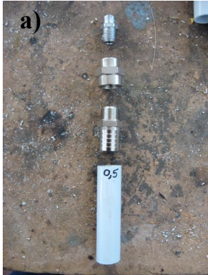
Figure 1. Nozzle line setup. (a) Nozzle assembly. The threaded pressure washing nozzle was connected to a short length of PVC pipe using two connectors. (b) Alternating angles of nozzles and pressure gauge used to regulate flow.
