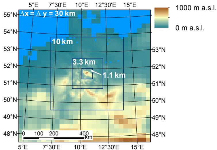
**Fig. 2.** WRF domains of the study area. The resolution of the first (outer) domain is 30 km, the fourth and final (inner) domain's resolution is 1.1 km, respectively.
