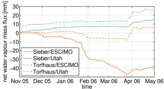
**Fig. 11.** Simulations of the net water vapour mass flux as calculated by ESCIMO and the Utah Energy Balance Model for the Sieber catchment and Torfhaus meteorological station. Positive values refer to a gain of water vapour due to condensation or resublimation whereas negative values indicate sublimation losses from the snowpack.
