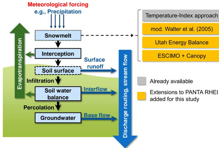
**Fig. 3.** Conceptualization of hydrological processes in PANTA RHEI (adapted from LWI-HYWAG and IfW, 2012). According to Sect. 2.4 each snowmelt model can be seen as alternative representation of the snowmelt processes.
