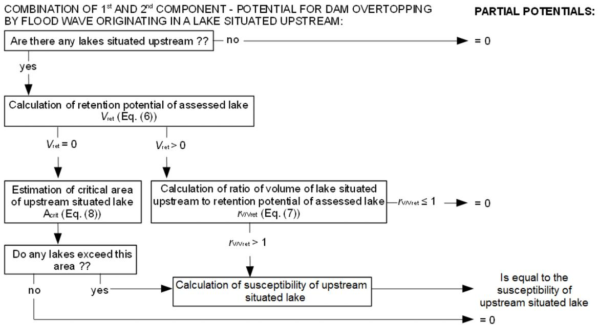
2Figure 2. Decision tree for assessing the potential for dam overtopping following a flood wave originating in a lake situated upstream (Scenario 2).
