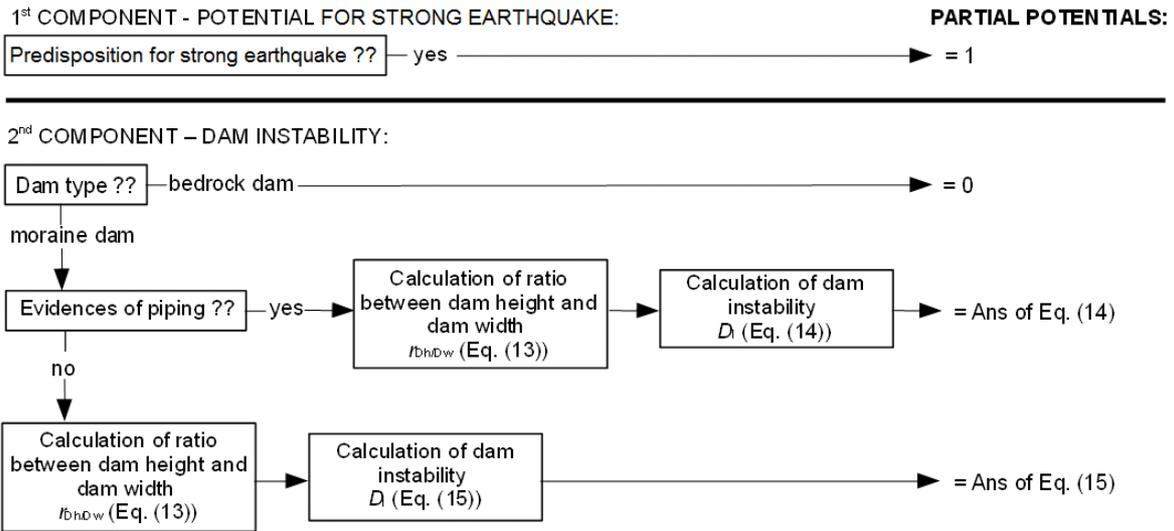
2Figure 5. Decision tree for assessing the potential for dam failure following a strong 3earthquake (Scenario 5).
