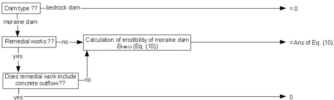
2Figure 3. Decision tree for assessing the potential for dam failure resulting from a fast slope
