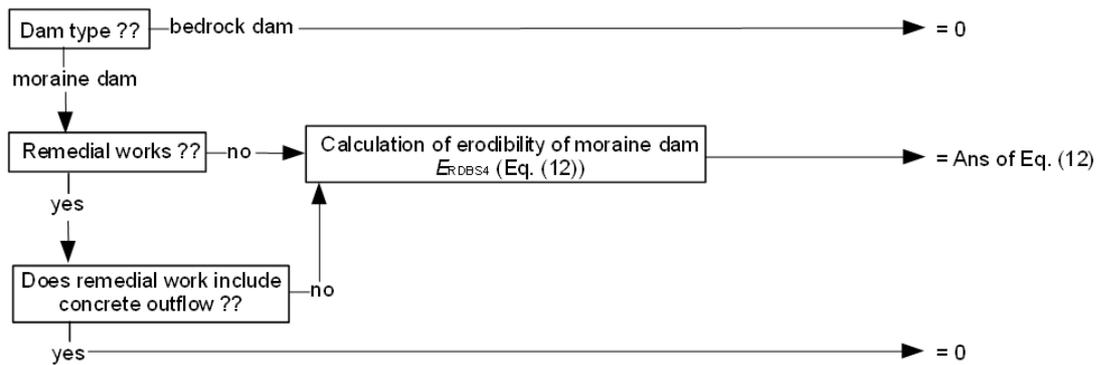
1Figure 4. Decision tree for assessing the potential for dam failure following a flood wave 2originating in a lake situated upstream (Scenario 4). The overall potential is derived as a 3product of three partial components.
