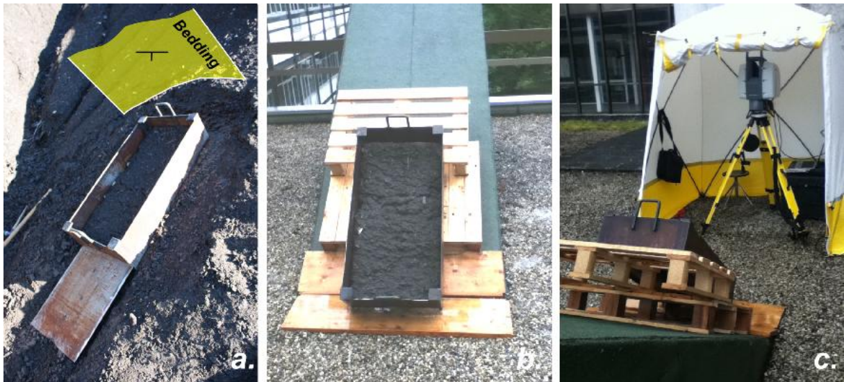
274 Figure 1: a. view of the sampling and the metal case (1 m x 0.5 m x 0.20 m) showing bottom 275 plate partially entered and the approximate orientation of the bedding. b: View of the sample 276 of soil inclined at 45° during the rainfall. c. Position of the TLS relatively to the metal case 277 which is protected from rainfall by a tent.
