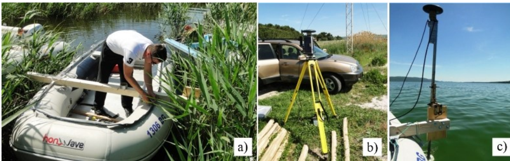
21 Figure 2. (a) Hondawave inflatable boat with wooden support. (b) Base GPS and UHF 22 antenna. (c) Rover GPS and dual-frequency probe
