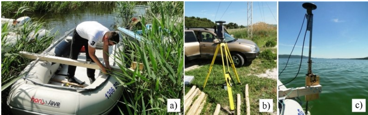
19 20 21 Figure 2. (a) Hondawave inflatable boat with wooden support. (b) Base GPS and UHF 22 antenna. (c) Rover GPS and dual-frequency probe
