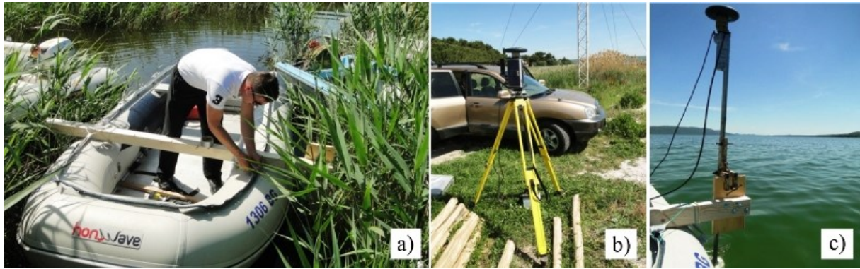
Figure 2. (a) Hondawave inflatable boat with wooden support. (b) Base GPS and UHF antenna. (c) Rover GPS and dual-frequency probe
