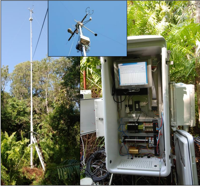
Fig. 3. (a) Telescopic mast (21.3 m) erected in the swamp forest to raise the eddy covariance instruments above the forest canopy, (b) the computer installed at the swamp forest, housed in a temperature controlled enclosure and (c) the instruments attached to the head of the mast.
