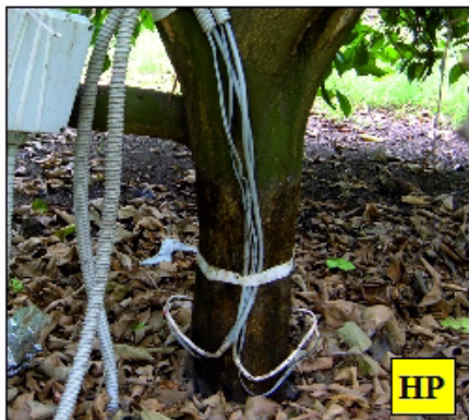
Figure 1. Bulgherano experimental site: the Eddy Covariance (EC) tower and a Heat Pulse (HP) Sap Flow installation on an orange tree.
