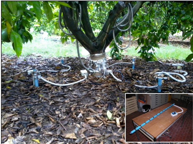
Figure 3. 3-D ERT apparatus installed around one orange tree. The system is composed of four micro-boreholes carrying 12 electrodes each (see inset) and 24 surface electrodes – see text and Fig. 4 for geometry details.
