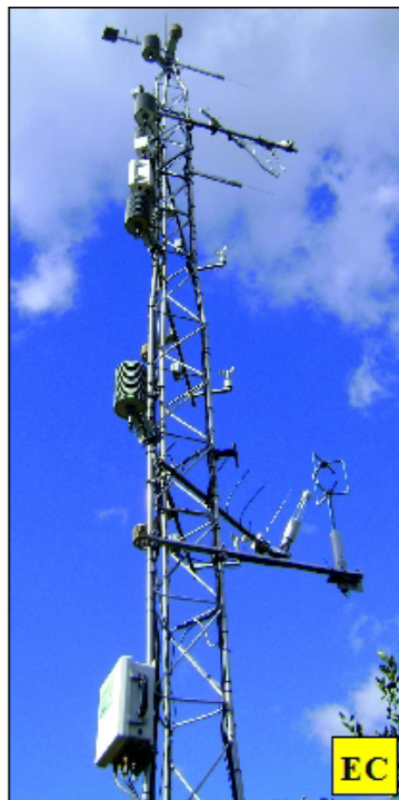
Figure 1. Bulgherano experimental site: the Eddy Covariance (EC) tower and a Heat Pulse (HP) Sap Flow installation on an orange tree.
