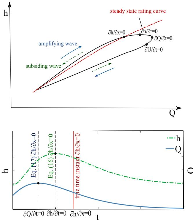
**Figure 2.** Comparison between rating curve for flood wave and steady flow with characteristic points, based on (Henderson, 1963) (upper panel), and impact of kinematic wave approximation (Eqs. 16 and 17) on the assessment of time instant at which  $\vartheta = 0$  (lower panel).
