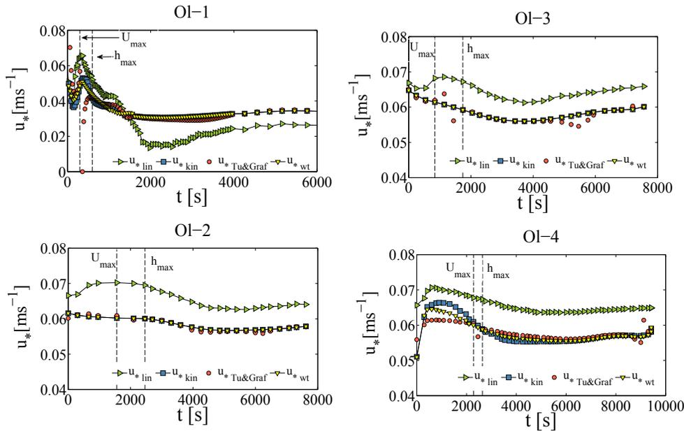
**Figure 8.** Comparison of friction velocity  $u_*$  evaluated by different methods (symbols defined in the text) for experimental flood waves in Olszanka River.
