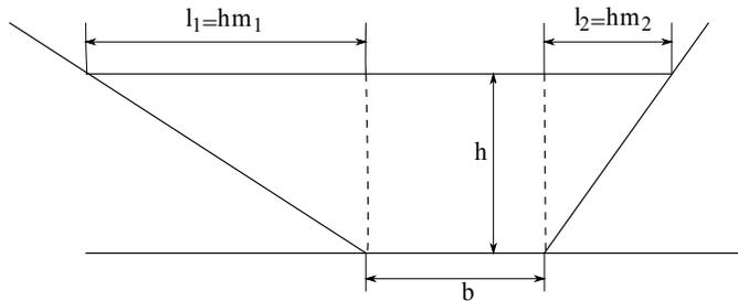
**Figure 1.** Trapezoidal cross-section of a channel with definitions of symbols used in the text.
