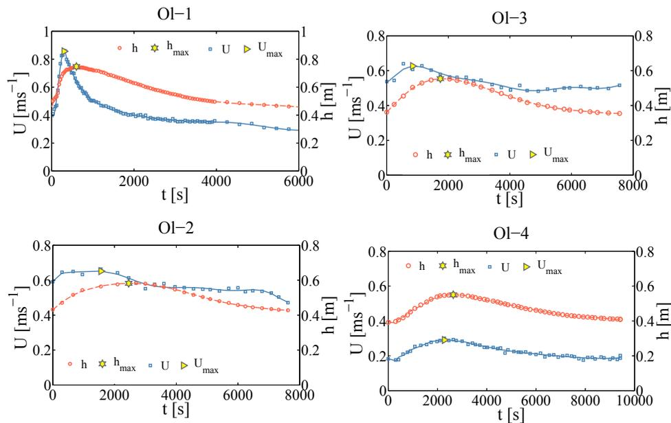
**Figure 4.** Temporal variability of flow depth  $h$  and mean velocity  $U$  for experimental flood waves in Olszanka River.
