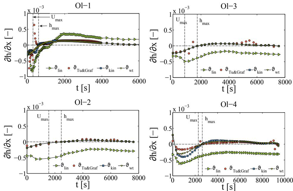
**Figure 6.** Temporal variability of gradient of flow depth  $\vartheta = \frac{\partial h}{\partial x}$  for experimental flood waves in Olszanka River.
