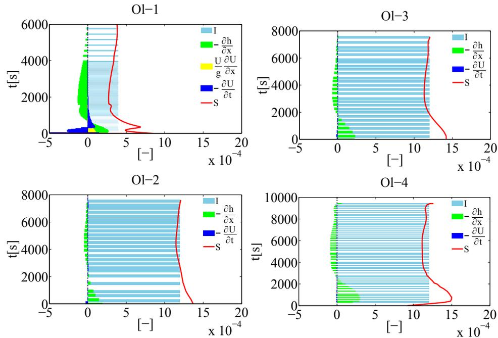
**Figure 7.** Comparison of terms of the momentum balance equation for experimental flood waves in Olszanka River.
