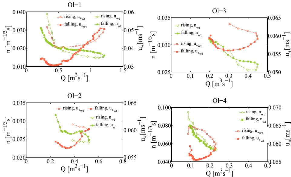
**Figure 11.** Comparison of the relation of Manning  $n$  vs. flow rate  $Q$  and friction velocity  $u_*$  vs.  $Q$  along rising and falling limbs of waves for experimental flood waves in Olszanka River.
