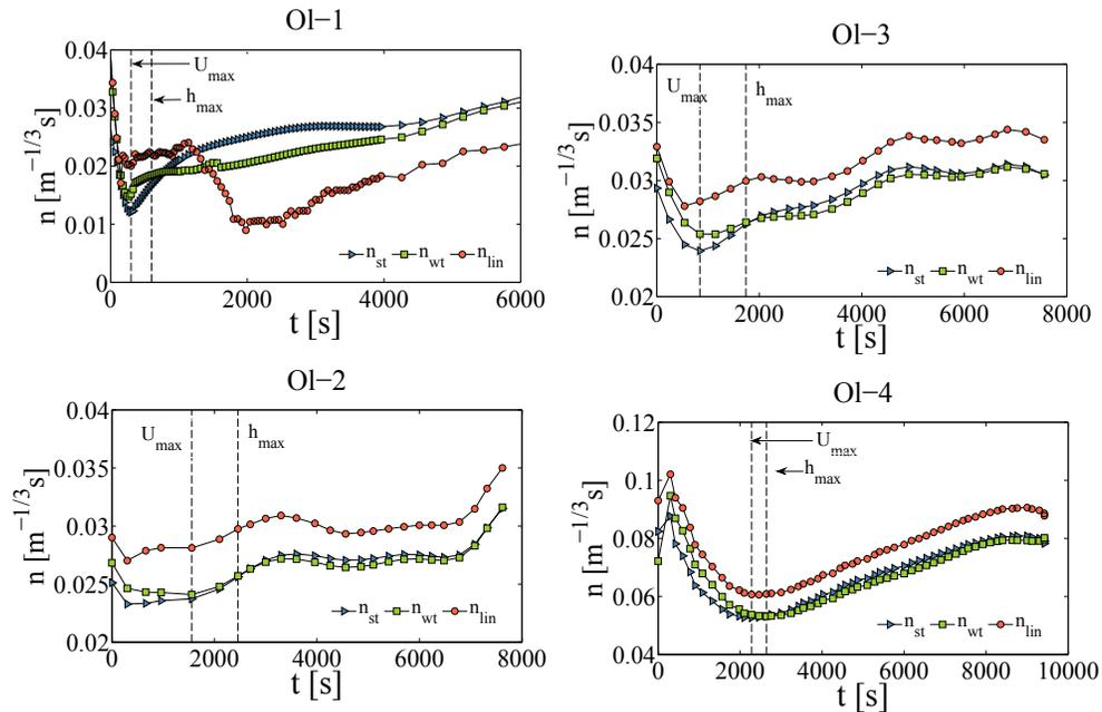
**Figure 10.** Temporal variability of Manning  $n$  evaluated for different assumptions about energy slope  $S$  for experimental flood waves in Olszanka River.
