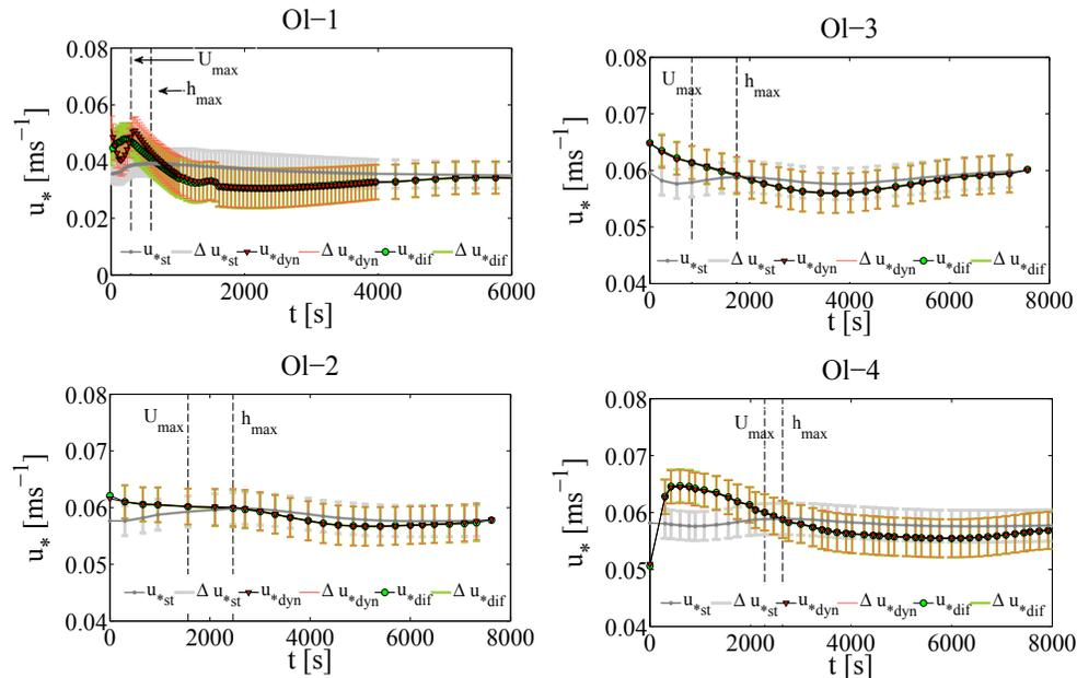
**Figure 9.** Comparison of friction velocity evaluated by formulae for dynamic  $u_{*dyn}$ , diffusive wave  $u_{*dif}$  and steady uniform flow  $u_{*st}$  with uncertainty bounds for experimental flood waves in Olszanka River.
