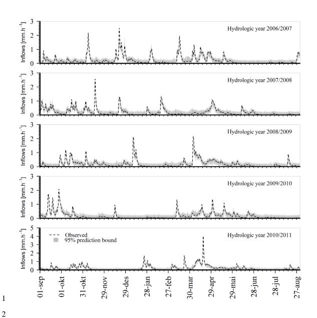
3 Figure 8. Observed hydrograph (broken lines) and the forecasted 95% confidence interval.
