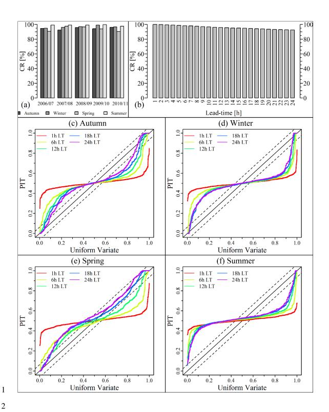
Figure 9. Reliability score (containing ratio-*CR*) for 95% prediction interval for: (a) each season of every hydrologic year; and (b) different forecast lead-times based on entire series. Panels (c)-(f): sample PIT uniform probability plots for each of the four seasons at 1, 6, 12, 18 and 24 hour forecast lead-times. Solid line designates the theoretical uniform distribution, broken lines represent the Kolmogorov significance band, and the dots denote PIT value of the observed p-values.
