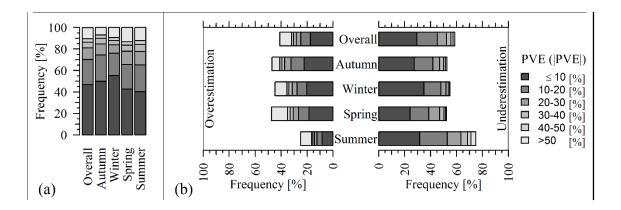
Figure 5. Stacked-column plots of: (a) PVE counts of the six absolute PVE classes ( $\leq$ 10%, 10-20%, 20-30%, 30-40%, 40-50% and >50%) observed in reservoir inflow forecasts from the complementary setup; and (b) the corresponding fraction of times under- and over-estimation incidents corresponding to the six PVE classes occurred. Hydrologic years 2006/07-2010/11.
