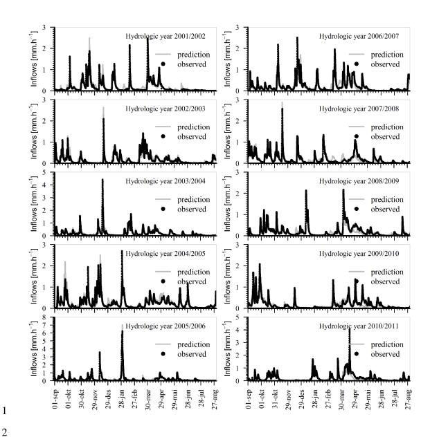
Figure 2. Observed and predicted reservoir inflow hydrographs during calibration (left column) and validation (right column) of the conceptual model.
