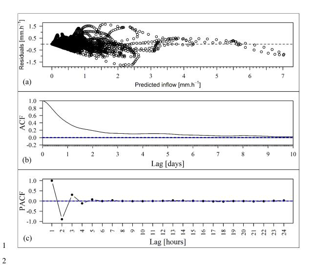
Figure 4. Plots of (a) residuals from the conceptual model as a function of predicted inflow during the calibration period, (b) autocorrelation function of the residuals, and (c) partial autocorrelation functions of the residuals.
