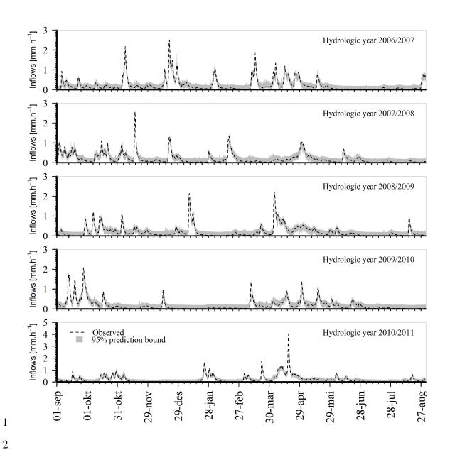
3 Figure 8. Observed hydrograph (broken lines) and the 95% prediction bound
