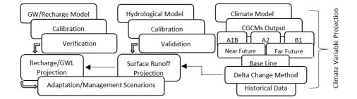
**Figure 3.** Flow chart showing the methodology used in this study to project climate change impacts on surface water and groundwater recharge/level in an arid region.
