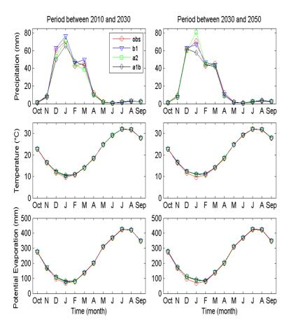
**Figure 4.** Mean monthly precipitation (mm), temperature (°C), and potential evaporation (mm) for historical climate data (1990–2010) relative to A1b, A2, and B1 scenarios for the periods 2010–2030 and 2030–2050.
