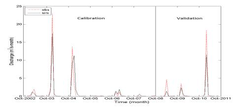
**Figure 6.** Observed and simulated monthly discharge (m<sup>3</sup> s<sup>-1</sup> month<sup>-1</sup>) for the Baba Arab discharge station from 1 October 2002 through 30 September 2011.
