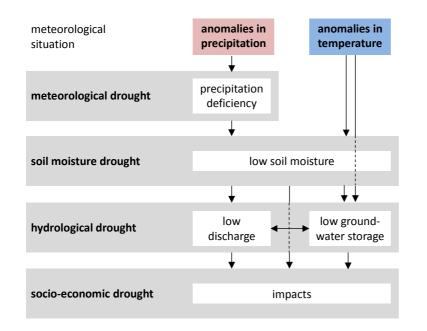
Figure 1. Scheme representing drought propagation (adapted from Fig. 8.1 of Van Loon, 2013).
