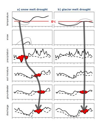
**Figure 3.** Synthetic time series representing the propagation of a meteorological anomaly (precipitation and/or temperature) through the terrestrial hydrological cycle for the new hydrological drought types (HDTs), (a) *snowmelt drought* and (b) *glaciermelt drought*. (Legend: see Fig. 2.)
