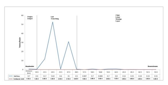
Fig. 10. The soil loss and sediment yield from headwaters to downstream (river mouth)
