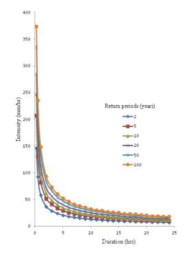
Fig. 1. IFD relationships of Dhaka City developed by Ahammed and Hewa (2012).
