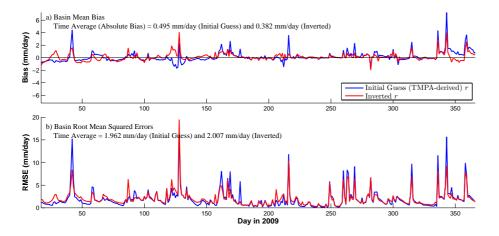
**Fig. 10.** Time series of basin mean bias **(a)** and root mean squared errors **(b)** from the Real Experiment using TMPA-derived runoff field as initial guess and real USGS gauge measurements. All lines are plotted the same way as in Fig. 7.
