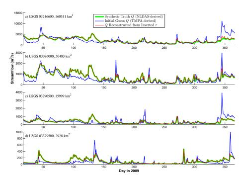
**Fig. 8.** Time series of streamflow estimates from the inversion experiment using TMPA-derived runoff as initial guess at 4 USGS gauge stations. Thick green lines are for the synthetic truth (NLDAS-derived), blue for the initial guess (TMPA-derived), and red for the streamflow reconstructed from the inverted runoff.
