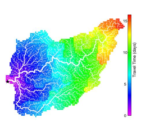
Fig. 2. Flow paths over the 0.125° grid and runoff travel time to the basin outlet.
