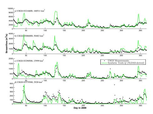
**Fig. 3.** Streamflow predictions from the routing model using the synthetically "true" NLDAS rainfall (green line) versus USGS measurements (black dots) over 4 gauge stations. The USGS gauge station number and drainage area is noted in the panel title.
