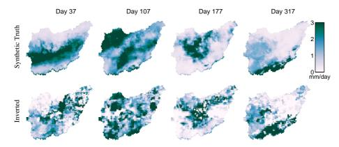
**Fig. 9.** Synthetic truth (NLDAS-derived) and inverted runoff fields for 4 days (Day 37, 107, 177, and 317 of 2009, same as Fig. 5) from the Real Experiment using TMPA-derived runoff field as initial guess and real USGS gauge measurements.
