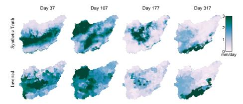
**Fig. 5.** Synthetic truth (NLDAS-derived) and inverted runoff fields for another 4 days (Day 37, 107, 177, and 317 of 2009) from the Synthetic Experiment using the null initial guess of runoff (constant field of  $1.474 \text{ mm day}^{-1}$ ).
