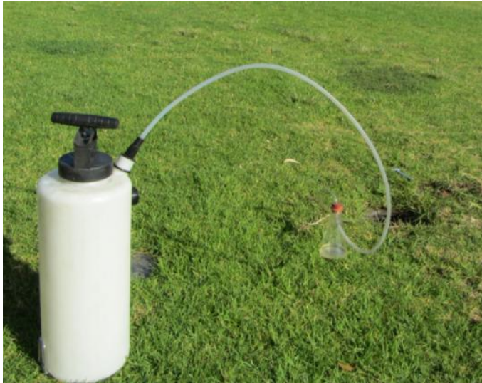
Fig. 3. Extracting water samples from a buried lysimeter.
