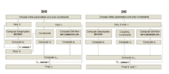
**Fig. 1.** Implementation of the SHI (left) and JHI approach (right).  $\pi$  and  $\gamma$  respectively indicate the geophysical and groundwater model parameters, where the bold formatted text mentions the specific software used in this paper.
