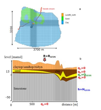
**Fig. 9.** Horizontal discretization of the Risby groundwater model and zonation of layer 1 (a) and the geological setup and boundary conditions used (b).
