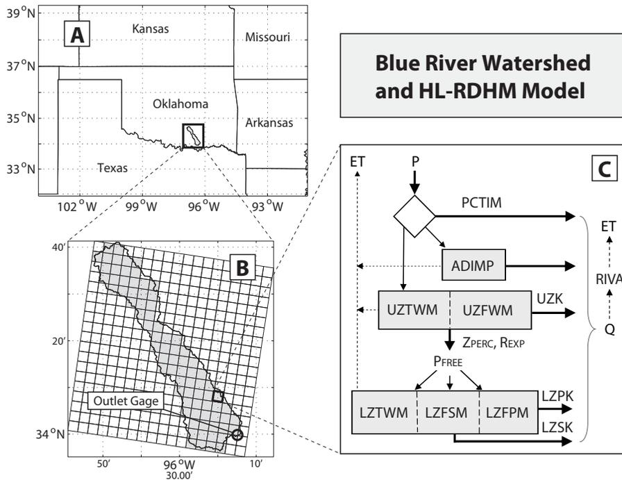
**Fig. 1.** (A) Location of the Blue River Basin in southern Oklahoma, USA. (B) The 78 HRAP grid cells of the Blue River Basin (shaded). (C) The Sacramento Soil Moisture Accounting (SAC-SMA) model, which simulates the water balance in each grid cell.
