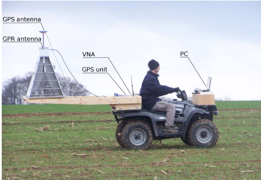
Fig. 3. All-terrain vehicle holding the GPR system constituted of the GPR horn antenna linked to a vector network analyzer (VNA), the GPS device, and the PC.
