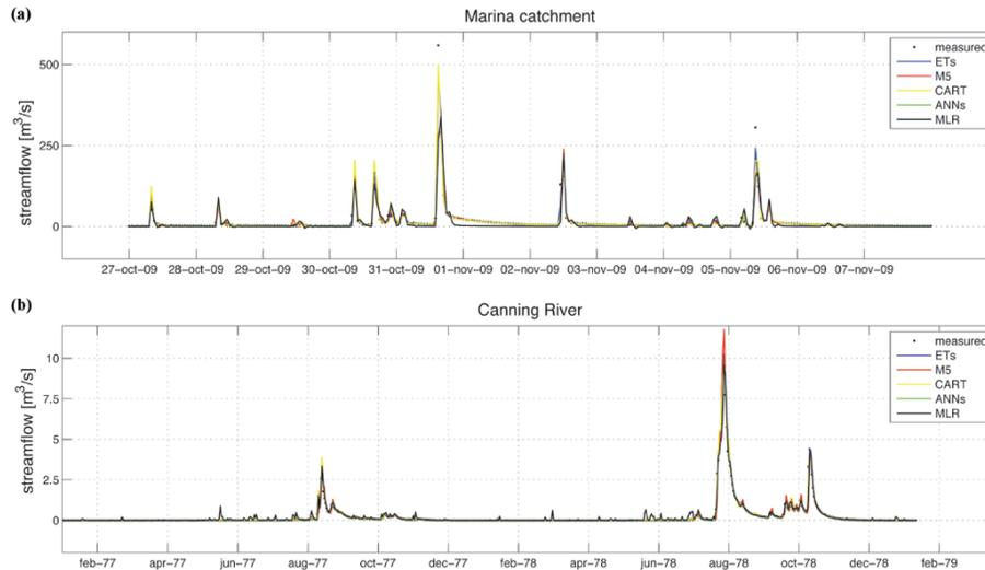
**Fig. 6.** Comparison between the measured and predicted streamflow for Marina catchment (a) and Canning River over the same period reported in Fig. 1.
