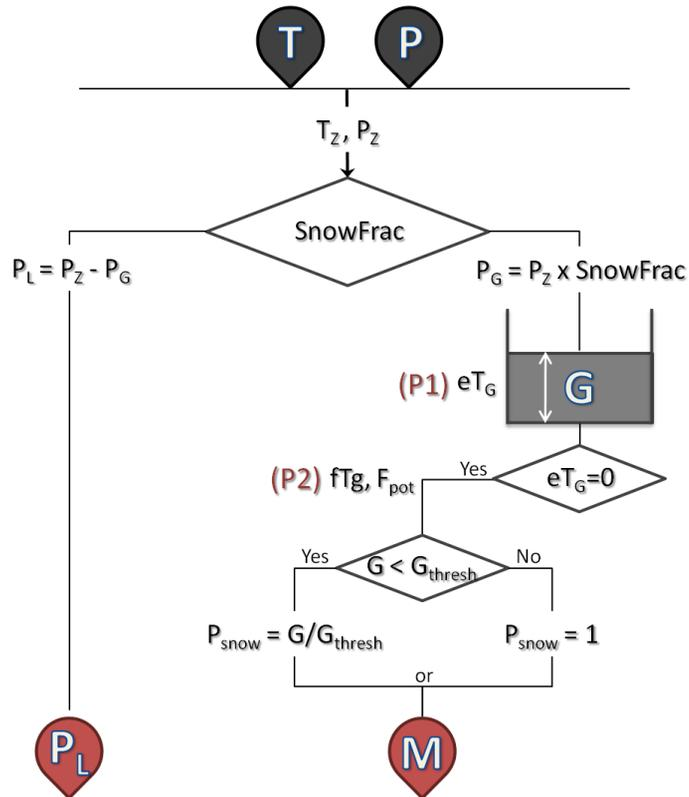
**Fig. 4.** Initial version of the CemaNeige snow module (N1).  $T$  is temperature,  $P$  is total precipitation,  $P_L$  is liquid precipitation, and  $M$  is snowmelt.  $G$  corresponds to the snowpack and  $P1$  and  $P2$  are the two free parameters (inspired from Valéry, 2010).
