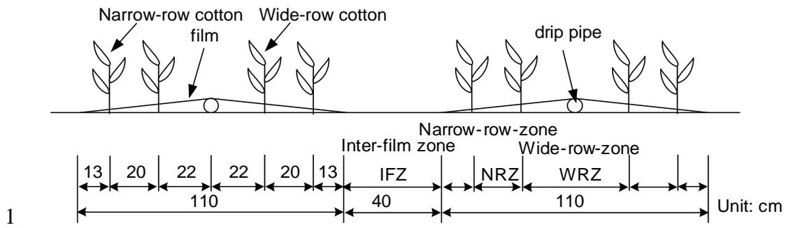
2 Fig. 2 One pipe, one film, and four rows of cotton arrangement
