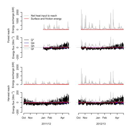
**Fig. 4.** Time series of hourly energy budget components (net radiation,  $Q_*$ ; latent heat flux,  $Q_e$ ; sensible heat flux,  $Q_h$ ; and heat addition due to friction,  $Q_f$ ) for the forest and harvest reaches for 2011/12 and 2012/13.
