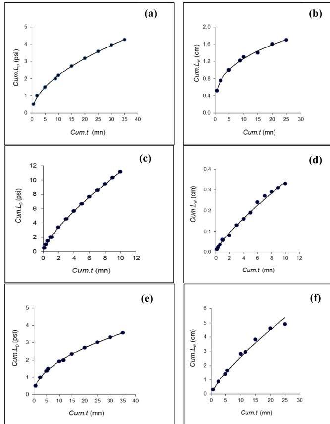
**Fig. 3.** Calibration of  $Cum.L_p$  using the curves of  $Cum.L_p$  vs.  $Cum.t$ ; **(a)** site-1 with  $R^2 = 0.9984$ , **(c)** site-2 with  $R^2 = 0.9981$  and **(e)** site-3 with  $R^2 = 0.9991$  and calibration of  $Cum.L_w$  using the curves of  $Cum.L_w$  vs.  $Cum.t$ ; **(b)** site-1 with  $R^2 = 0.9984$ , **(d)** site-2 with  $R^2 = 0.9967$  and **(f)** site-3 with  $R^2 = 0.9966$ , where the correlations are evaluated through power regression analysis.
