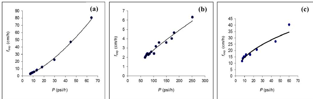
**Fig. 4.** Curve  $f_{th} = \alpha \times P^\beta$ ; **(a)** site-1, **(b)** site-2 and **(c)** site-3.
