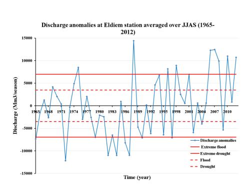
**Fig. 5.** The discharge anomalies at Eldiem station averaged over JJAS (1965–2012), the red line represent the threshold for the extreme flood/drought, and the dashed red line represents the threshold for drought/flood.
