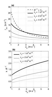
Fig. 4. (a) Additional aerodynamic resistance ( $r_{\rm a.c.}$ ) given by Eq. (20) is plotted as a function of wind speed at reference height  $(u_a)$  for different LAI and compared with the rough estimate based on  $B^{-1} = 4$ ; **(b)** the bulk parameter  $kB^{-1}$  (inferred from the value of  $r_{a,c}$ ) is plotted as a function of  $u_a$  for different LAI ( $L_t$ ).
