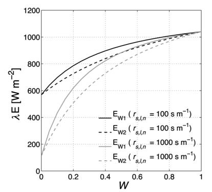
**Fig. 3.** Latent heat flux  $(\lambda E)$  from a partially wet canopy as a function of its fractional surface wetness (W). Comparison of two formulations for two different values of the minimal stomatal resistance  $r_{s,l,n}$  representing the canopy water stress:  $E_{W1}$  is the general formulation given by Eq. (28);  $E_{W2}$  is the simplified formulation given by Eqs. (33) and (34). Soil surface resistance  $r_{s,s}$  is set to  $500 \, \mathrm{s} \, \mathrm{m}^{-1}$ .
