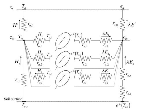
**Fig. 1.** Resistance network and potentials for a canopy represented by its elementary exchange surfaces (see list of symbols). All the component fluxes (sensible heat  $H_i$  and latent heat  $\lambda E_i$ ) converge at canopy source height  $(z_m)$ .  $T_{c,s}$  is soil surface temperature.
