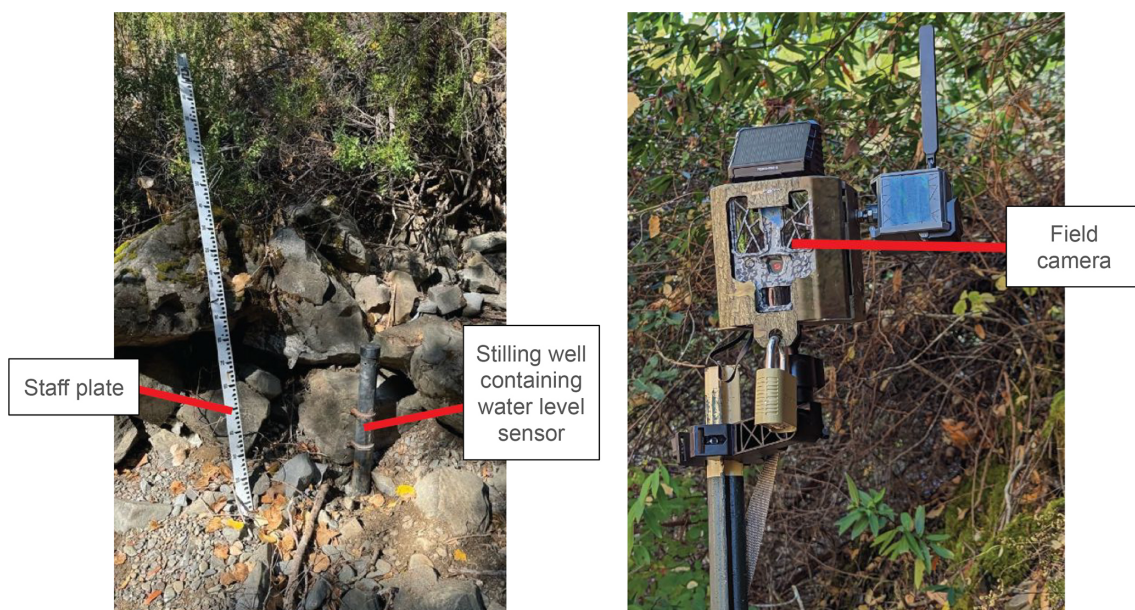
Figure 2. Perry Creek (PEC) streamgage station equipment. The staff plate, stilling well, and water level sensor (left) are located at the side of the streambed; the field camera (right) is located across the stream channel, facing the staff plate.
